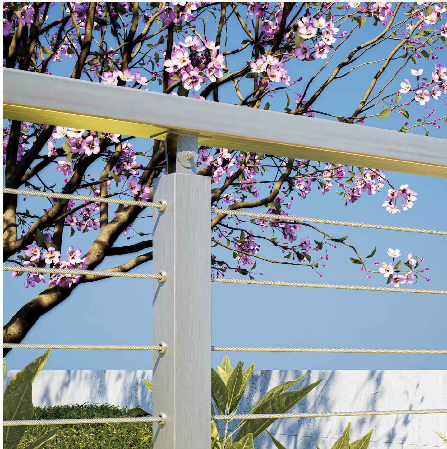
The image shows a 316 stainless steel pre-fabricated 2" square cable rail post system, 36" in height, featuring a fixed flat handrail saddle, 1/8" 316 stainless steel cable kit, and 2205 duplex stainless steel handrail with 1-1/2" fittings.
